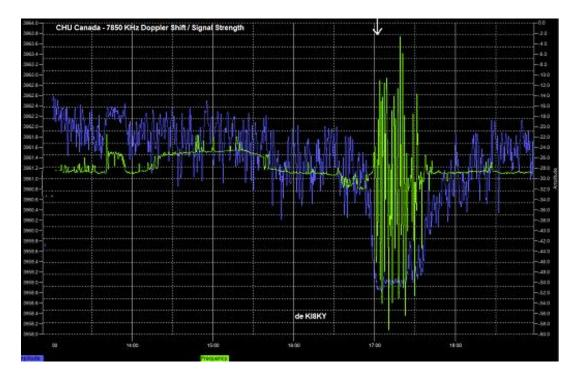
"I monitor the frequency and field strength of Canada's CHU time station transmitting at 7850 KHz," explains Curtis. "During the X-class flare event, I was able to detect the Doppler shift of the station's carrier frequency (green plot). It shifted by 5 Hz, which is a small change, but very obvious!"
